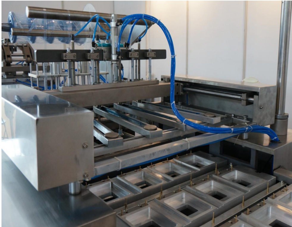
No.4 Blister Spreading Station
